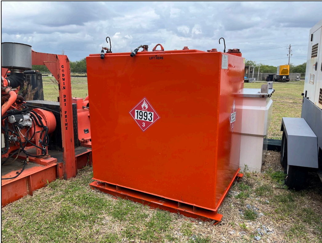
35. A fuel storage container in the storage area from the previous photo can be seen. The container appears to be used for diesel.
